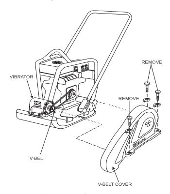
Figure 7. V-Belt Cover Removal
